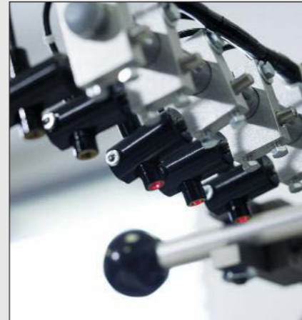
Accurate positioning with the help of the 5 position lamps
